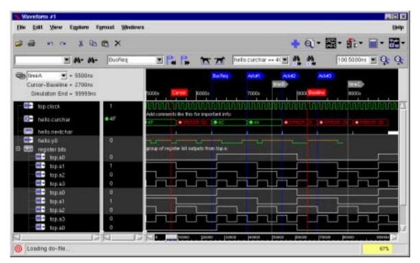
Figure 1: Main window of the SignalVision waveform plotting tool. The tool is a mixture of custom-built widgets, BLT widgets, and [incr Tcl/Tk] mega-widgets, all stitched together with Tcl code.
